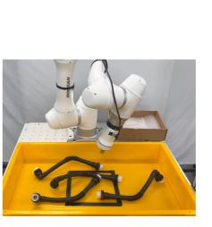
An optional built-in Fail Safety Function ensures that the gripped object is not lost even when the power is cut off.
